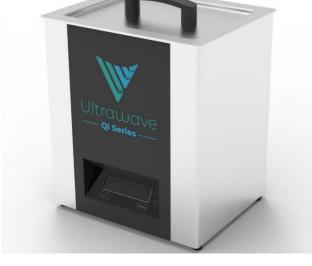
The Qi-200 is a 12Litre ultrasonic cleaner with a menu driven, LCD control panel. This allows simple adjustment of cycle time (0 to 99mins or infinity mode), temperature (ambient to 80°C), ultrasonic power and frequency mode for precise and accurate processing.
